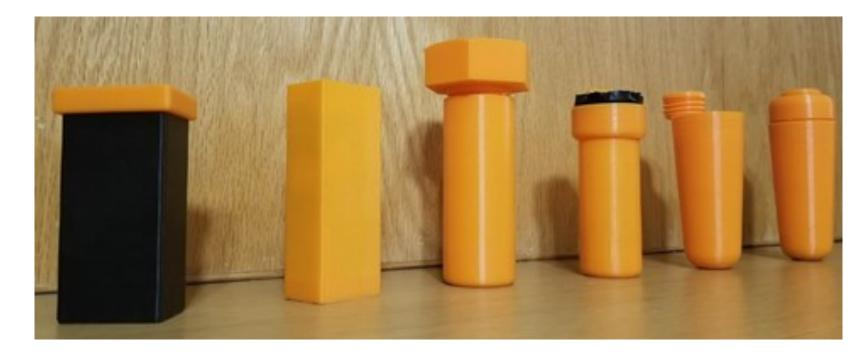
As we gained familiarity with CAD the encapsulation design progressed and increased in complexity. The result is a sleek three-piece threaded structure that makes testing and calibration a lot easier. The final structure shown has room to put weights (quarters) in both the top and bottom sections to vary the center of gravity and overall mass of the hydrometer.
